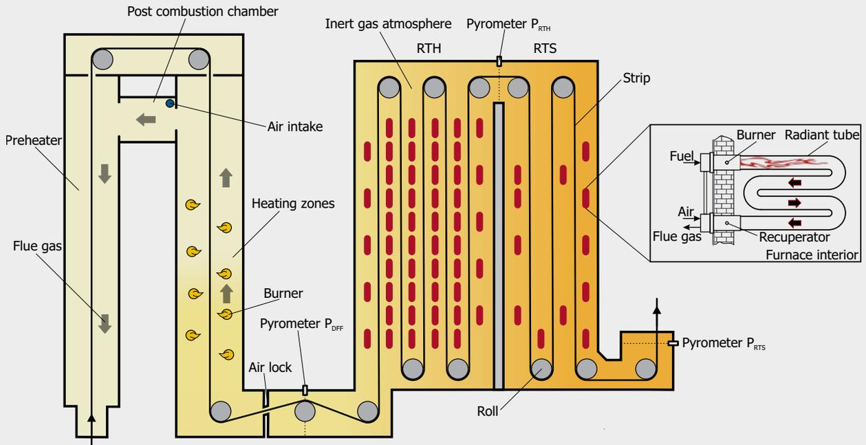
**Fig. 1:** Combined direct- and indirect-fired strip annealing furnace
