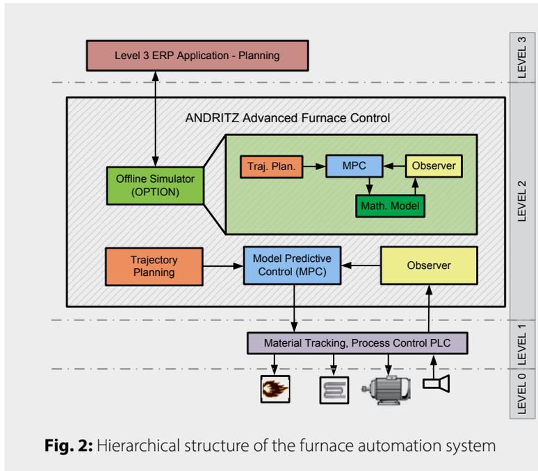
**Fig. 2:** Hierarchical structure of the furnace automation system
